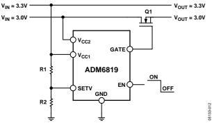
Figure 18. ADM6819 Applications Diagram
