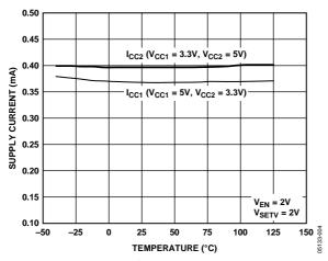
Figure 8. Supply Current vs. Temperature
