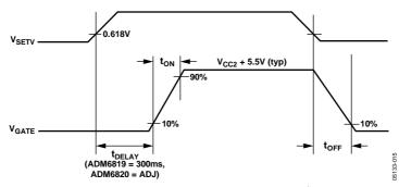
Figure 3. ADM6819/ADM6820 Timing Diagram Using SETV for Sequencing
