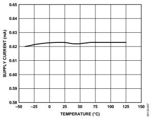
Figure 11. Supply Current vs. Temperature
