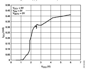
Figure 9. I<sub>CC2</sub> vs. V<sub>CC2</sub>
