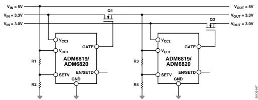
$\textit{Figure 5. ADM} 6819 / \textit{ADM} 6820 \, \textit{Solution for Sequencing Three Supply Rails}$
