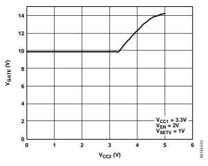
Figure 14. V<sub>GATE</sub> vs. V<sub>CC2</sub>
