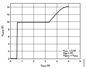
Figure 12. V<sub>GATE</sub> vs. V<sub>CC2</sub>
