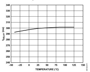
Figure 15. t<sub>DELAY</sub> vs. Temperature
