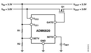
Figure 19. ADM6820 Applications Diagram
